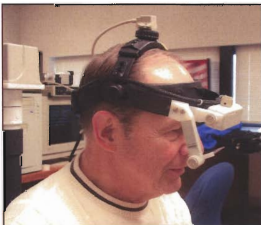
Figure 6 [35] : Eye and Head tracking system
